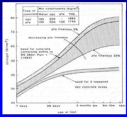
Strength development with additional fly ash in concrete mixes
