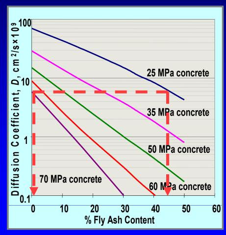
For equal chloride diffusion coefficient:
